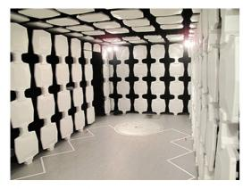
The SpaceSaver™ 26H is an RF-shielded semianechoic chamber providing a multi-purpose environment for radiated immunity and precompliant emission testing. This compact chamber provides an anechoic test environment that supports testing up to 40 GHz with anechoic performance equal to or better than that required for radiated immunity testing per most standards including IEC, pre-compliant emission testing, and
