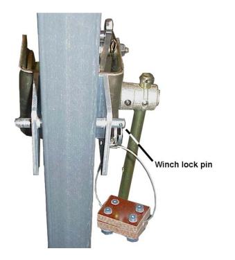
• Secure winch with winch lock pin by sliding the pin through the winch and mast.
