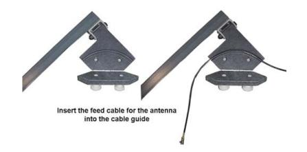
**9. Thread cable through cable guide**—Insert the feed cable for the antenna into the cable guide to reduce stress on the cable and antenna connector.
