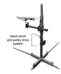
The mast is constructed of a high density fiberglass reinforced polymer with a high degree of immunity to structural deterioration from environmental elements. The base is an aluminum four-leg design for maximum support and portability. The design of the Model 1052 allows easy assembly and usage.
