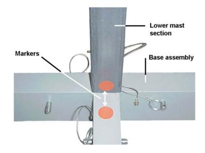
1. Attach lower mast section to base assembly—Install the lower mast onto the center post of the base assembly, aligning the markers.
