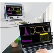
students can make measurements from their dorm room or other remote location with an exact replica of the oscilloscope screen in their browser.
