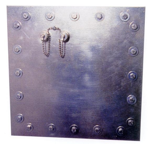
The material of the panel is of 3 mm galvanized steel and the collar frame is of 8 mm galvanized steel with threaded holes. The external dimensions of the complete panel are: clear opening dimensions + 80 mm.
