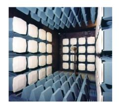
ETS-Lindgren's SpaceSaver™ FAR chambers are designed to perform IEC 61000-4-3 compliant radiated immunity measurements. Fully anechoic, these chambers can also be used for CISPR 16-1-4 pre-compliant radiated emissions measurement prescans, with fixed height. Frequency ranges for this chamber are 26 MHz to 40 GHz (radiated immunity) and 30 MHz to 40 GHz (radiated emission).
