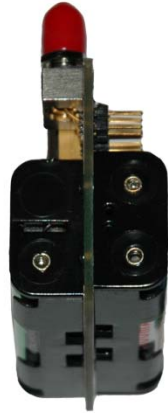
Vertical board with four batteries
