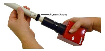
Position the alignment arrows on the probe and housing so they are lined up, and then gently press the probe into the housing.
