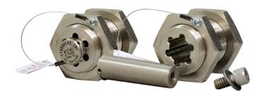
ing the enclosure's radio frequency isolation integrity. The filter has a removable center plug, which is surrounded by six waveguide bores. When the center plug is removed, connectorized fiber optic cables can be inserted into the peripheral cable sized slots.
