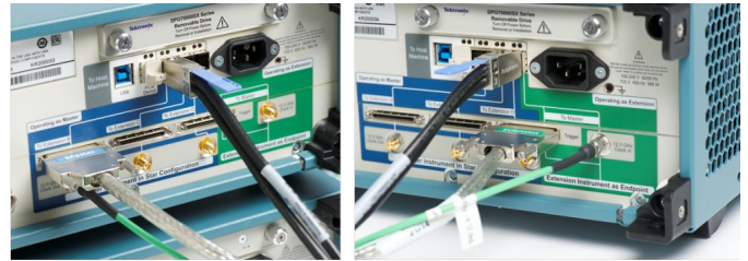
UltraSync connection on instrument with Master role
