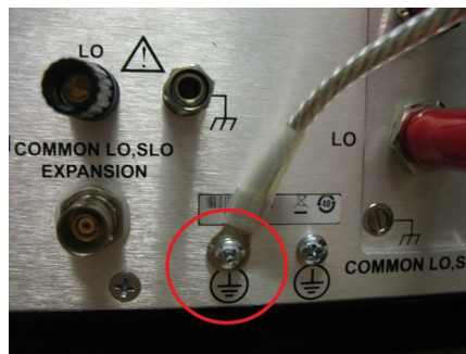
Figure 37: 8020-DP connected to protective ground
