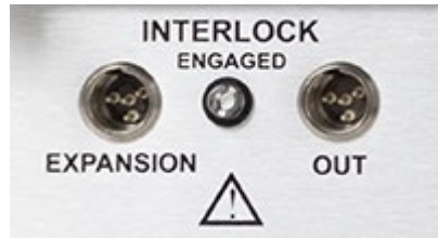
Figure 8: 8020 device side interlock connections
