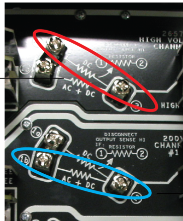
Figure 22: Model 8020 motherboard resistor between nodes 1 and 2
