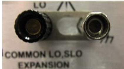
Figure 24: LO connector connected to chassis ground lug
