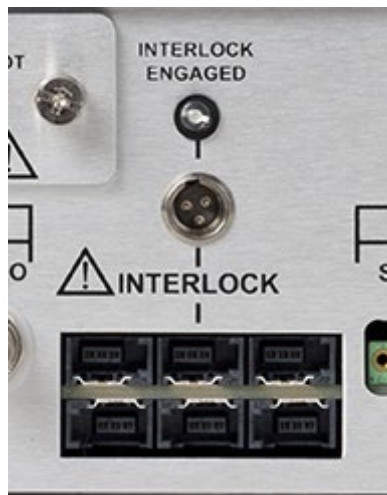
Figure 7: Instrument side interlock connectors
