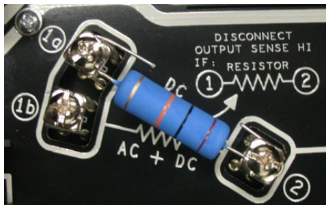
Figure 19: Resistor installed between nodes 1a and 2
