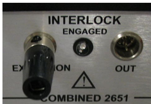
Figure 9: 8020 interlock plug installed
