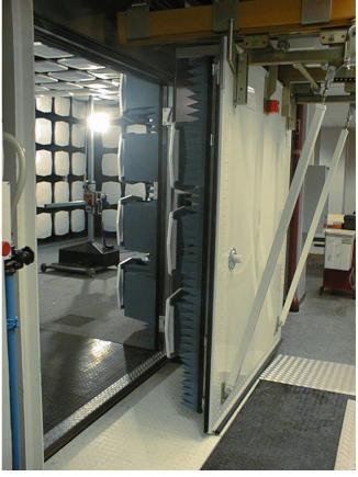
The door leaf of Euroshield RFSD-F/A-100 sliding doors is painted on outside (standard color white RAL 9010). Max. size for this door type is 3 m x 3 m (h).
