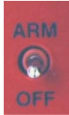
The ARM/OFF switch activates and deactivates the probe. In the ARM position, the probe is powered by its internal 3.6 VDC NiCd battery; in the OFF position, the probe is inactive. To prolong battery life, set the ARM/OFF switch to OFF at the end of a test sequence or when the probe is not in use.
