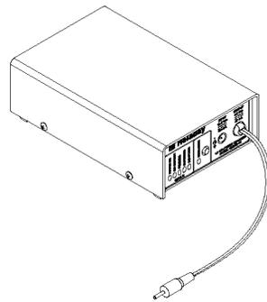
The H-491198-36 Nickel-Cadmium (NiCd) Battery Charger is a dual power source battery charger. It charges 3.6 volt 1400 mAH NiCd batteries and is powered by 120-240 VAC line power or 12.5 VDC. The H-491198-36 Battery Charger uses a  $-(dV)/(dT)$  negative delta V technique to determine when the battery is fully charged, which is typically one hour. With this technique, the charge state of the battery has no effect other than shortening the charge time.
