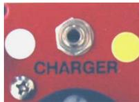
Each HI-4433 probe contains a rechargeable nickel-cadmium (NiCd) battery. A fully-charged battery (nominal output voltage of 3.6 VDC) provides up to 17 hours of continuous operation.
