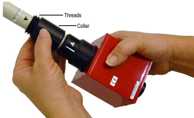
Pull the collar on the housing up to the threads on the probe and twist to begin tightening.
