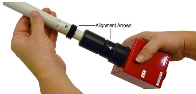
Position the alignment arrows on the probe and housing so they are lined up, and then gently press the probe into the housing.
