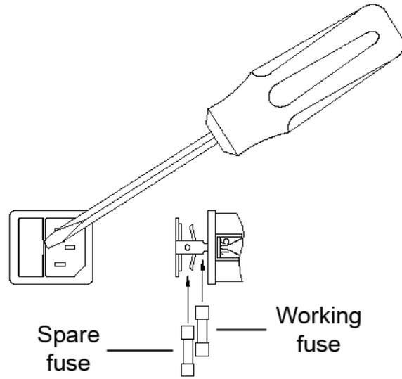
5. Replace the blown fuse with the spare fuse.
