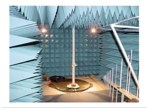
ETS-Lindgren's SpaceSaver<sup>™</sup> PC is a semi-anechoic chamber, designed to perform ANSI C63.4/CISPR 16-1-4 and IEC 61000-4-3 pre-compliant radiated immunity measurements. This chamber can also be used for ANSI C63.4 pre-compliant radiated emissions measurement prescans, with limited height scan. Frequency ranges for this chamber are 80 MHz to 40 GHz (radiated immunity) and 30 MHz to 40 GHz (radiated emission).
