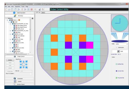
ACS maps devices and tests to sites and subsites, eliminating the need to duplicate each test for each subsite and reducing test development time.
