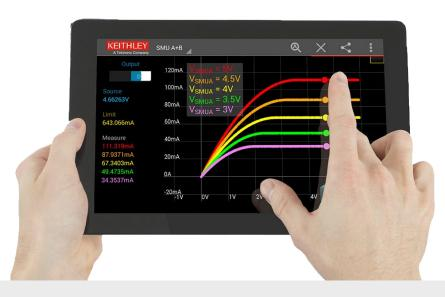
The IVy Android App works with Series 2600B SourceMeter® SMU Instruments to perform I-V characterization. Pinch and zoom for deeper insight into device performance.
