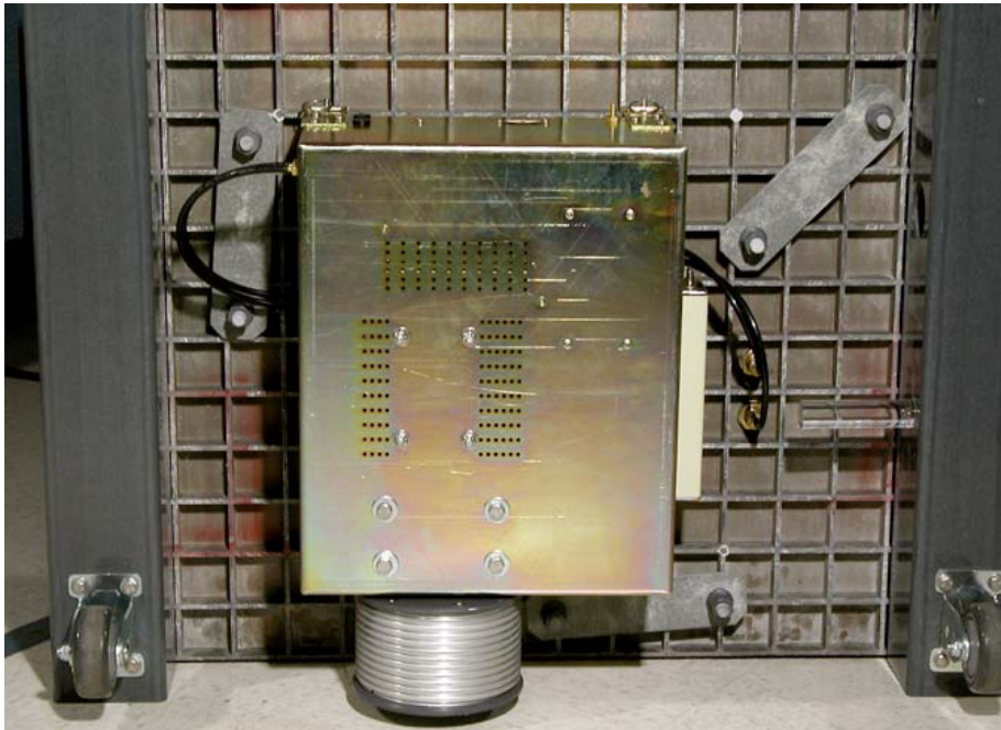
Figure 2: Motor attached to bottom of MiniMast
