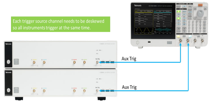
Figure 6: Setup diagram to quickly achieve moderate skew among channels
