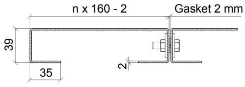
A standard panel size is 1120 mm x 3040 mm and the maximum size is 1120 mm x 4000 mm. For special purposes the panels can be tailor-made to any size and shape (non-standard treatment, e.g. welding might be required). Possible nominal lengths / widths in mm of a standard panel are:
