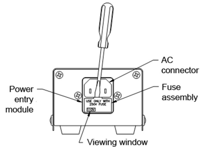
Check the viewing window on the power entry module to verify that the battery charger is set to the proper voltage for your AC power source. To change the voltage setting:
