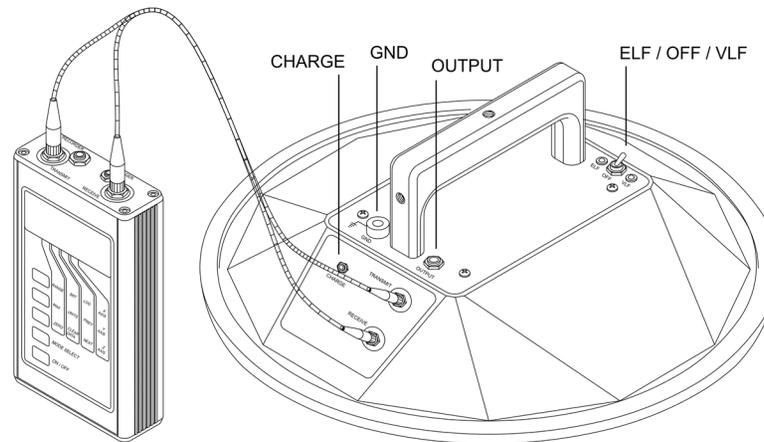
Attach fiber optic cables to TRANSMIT and RECEIVE connectors, matching white to white and yellow to yellow
