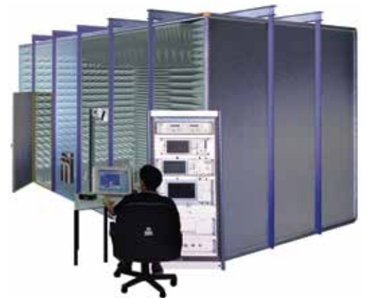
AMS-8100 Test System shown with optional equipment, including MAPS positioner upgrade.
